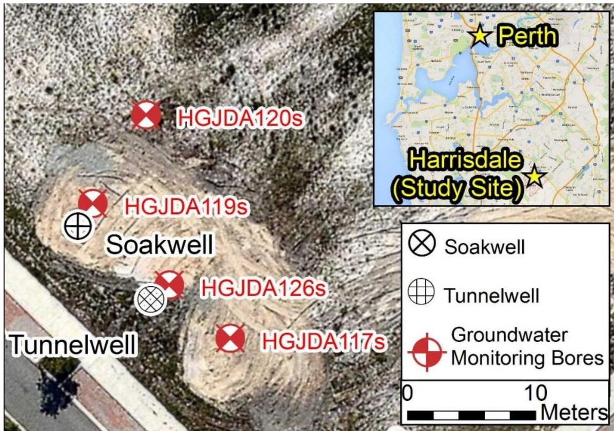
Figure 10: Experimental layout of soakwell, Tunnelwell and monitoring bores.
