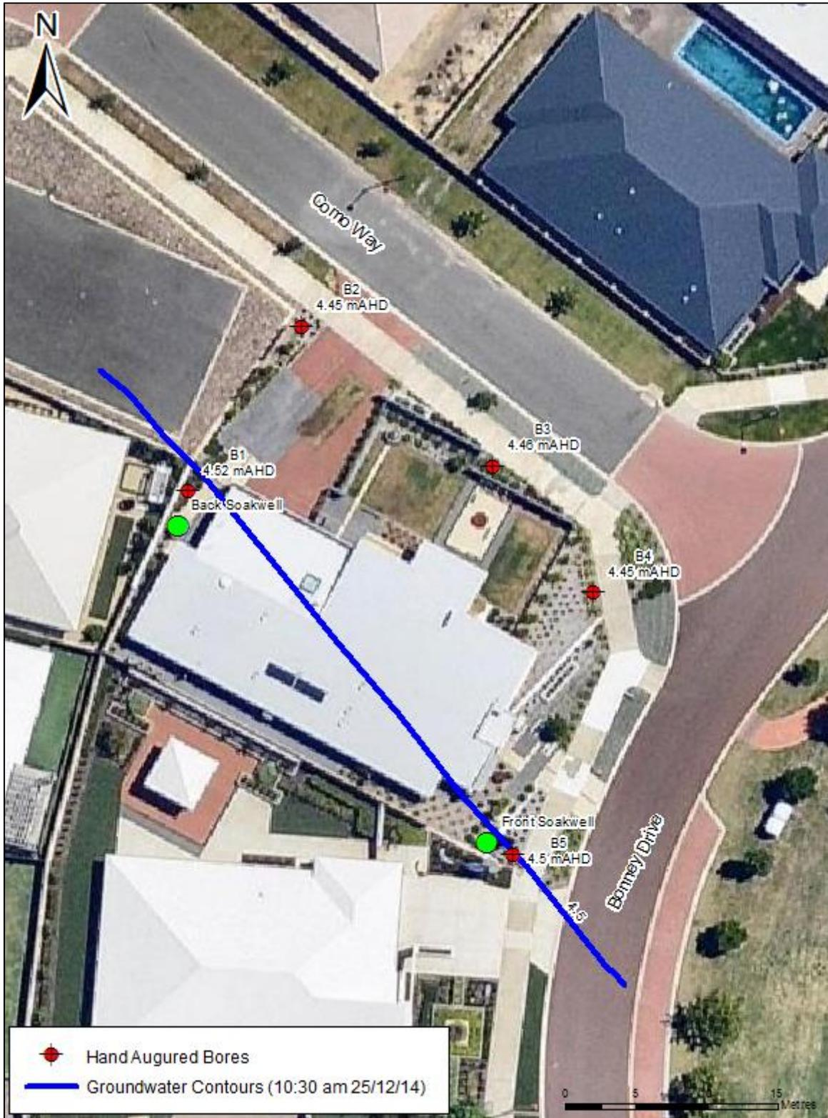
Figure 8: Groundwater Levels (10:30am 25/12/14)
