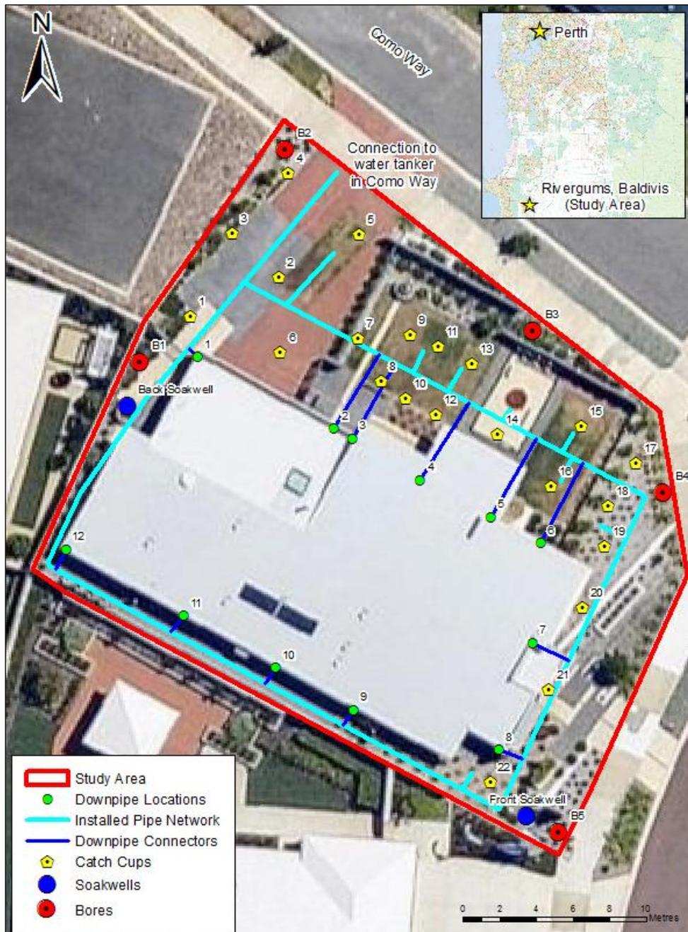
Figure 1: Location Plan and Experimental Layout
