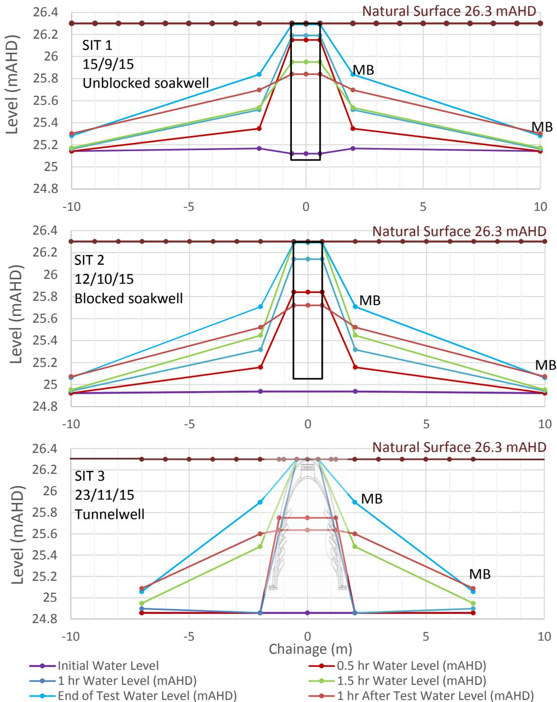
Figure 13: Cross sections of unblocked soakwell SIT 1 (top), blocked soakwell SIT 2 (middle) and Tunnelwell SIT 3 (bottom). MB = monitor bore.
