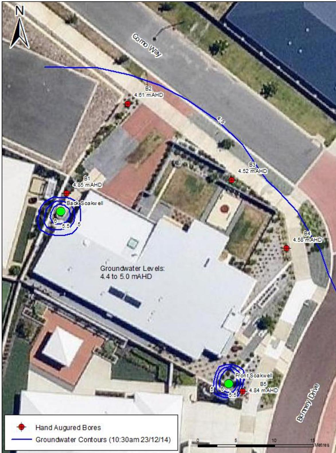
Figure 7: Groundwater Levels (10:30am 23/12/14)
