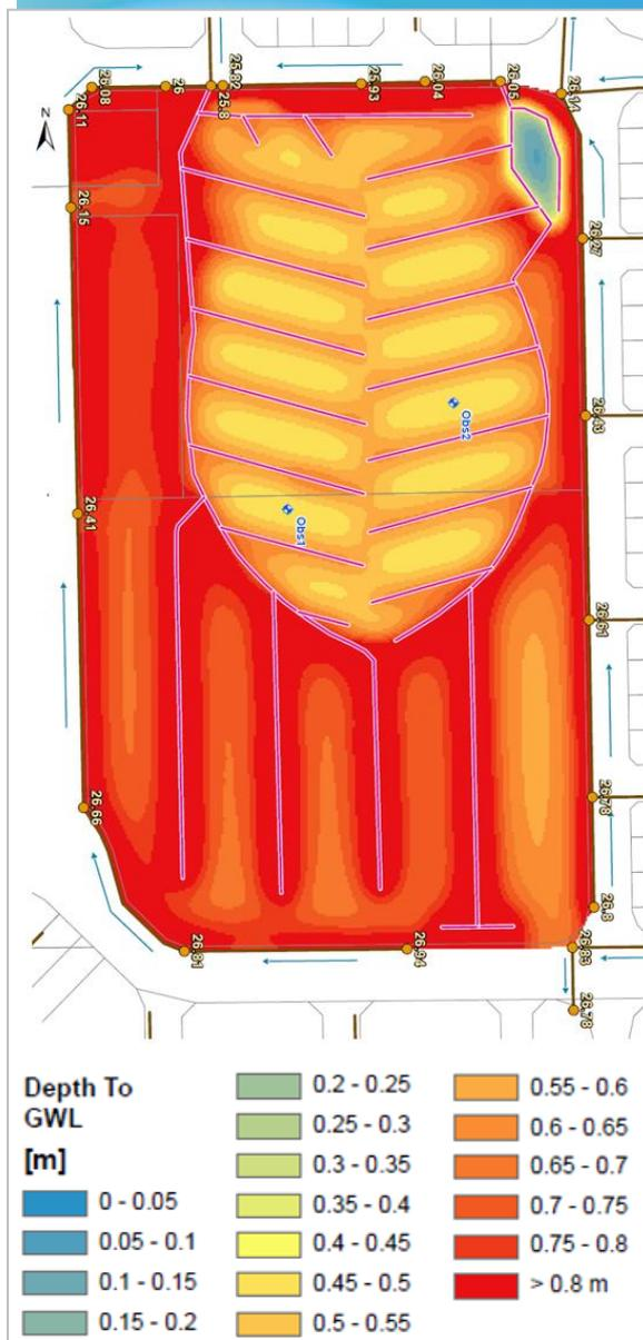
**Figure 9:** Case Study 2 – Depth to 20% AEP Groundwater Level
