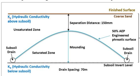
Figure 3: Schematic showing groundwater mounding between subsoil drains for Case Study 1.
